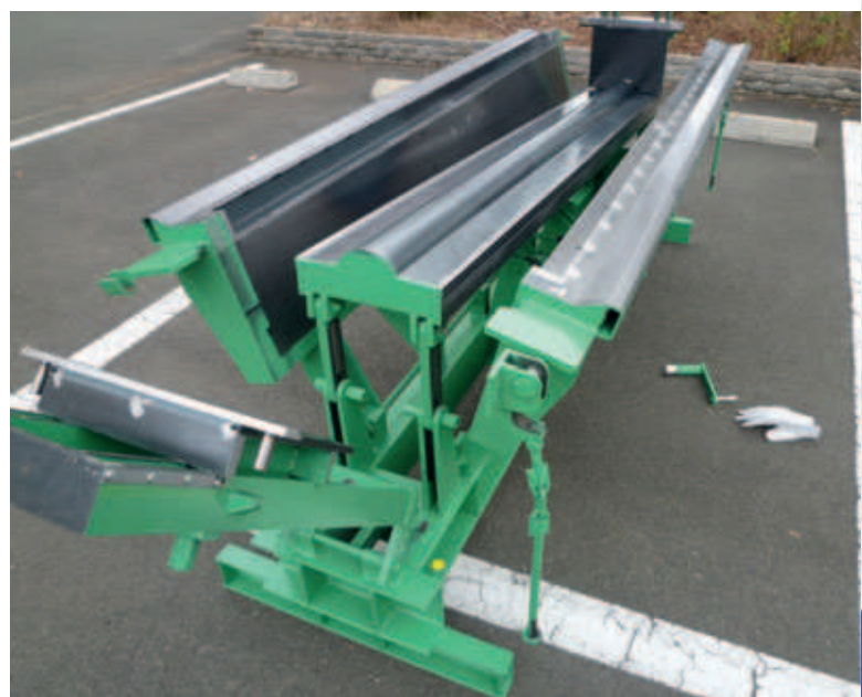
Fig. 2, 3: Since dimensioning is accomplished in the mould itself, changes in thickness are easy, mistakes are easy to avoid, and direction changes in slope are possible as well
