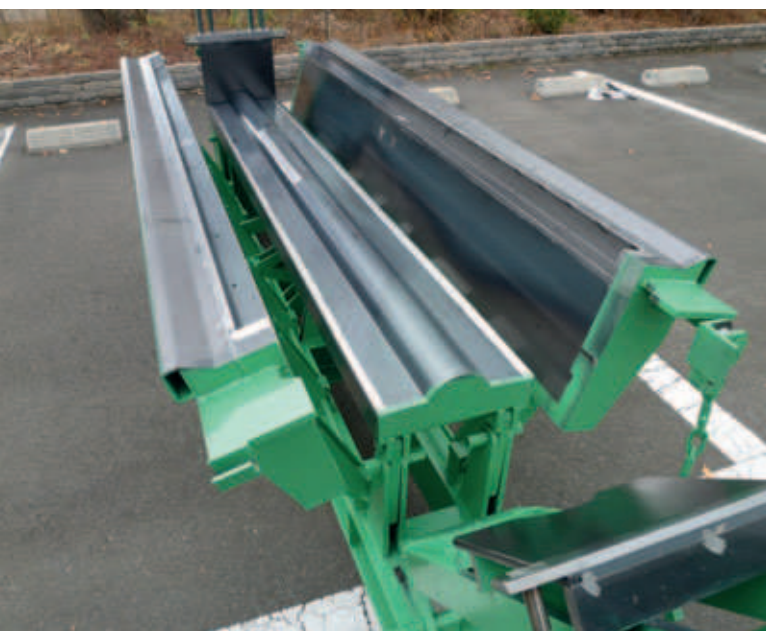
Fig. 2, 3: Since dimensioning is accomplished in the mould itself, changes in thickness are easy, mistakes are easy to avoid, and direction changes in slope are possible as well
