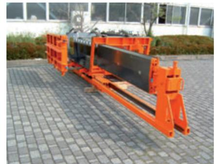
Fig. 3: The inner core is hung from one side with sliding rail
