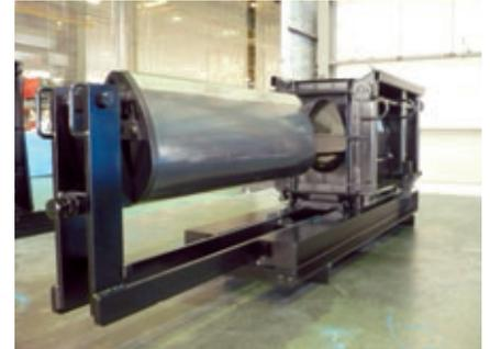
Fig. 2: Mold with roll-back type inner core
